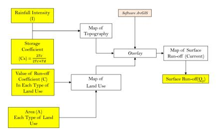
Figure 3. Flow Analysis of Surface Runoff Discharge Calculation in the Lesti Subwatershed
