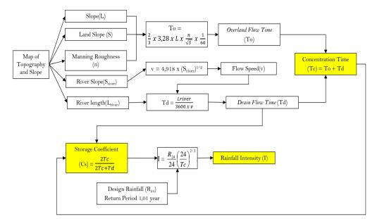
Figure 2. Flow Analysis of Concentration Time (Tc), Reservoir Coefficient (Cs) and Rain Intensity (I)
