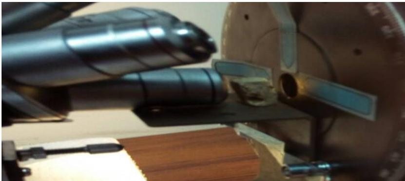
**Figure 5.** Microscope for measuring contact angle
