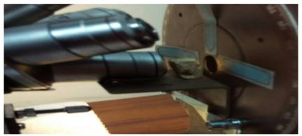
Figure 5. Microscope for measuring contact angle
