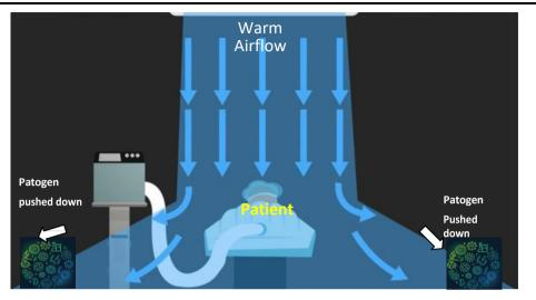
Figure 4. Warm and sterile vertical downward airflow in the patient room
