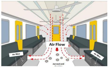
**Figure 2.** The ceiling fan's airflow can suppress virus-contaminated droplets and aerosols to fall to the floor immediately so that the room can be cleaner from aerosols and droplets. The dotted line shows the airflow line.
